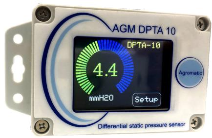
The DPTA 10 can be set to show the following measuring as full scale: 0 to 5 mm or 0 to 10 mm water column.
