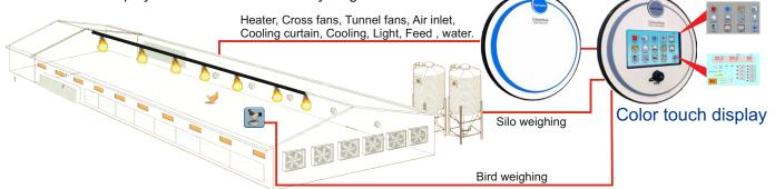
The Columbus AGM 10 climate controller can be ordered for various application as a OEM product . To the Columbus AGM20 Basic the following equipment can be connected.
