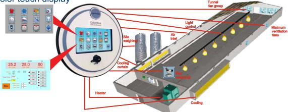
The Columbus AGM 10 climate controller can be ordered for various application as a OEM product . To the Columbus AGM10 Advance the following equipment can be connected. Up to 2 Silo weigher, 2 bird weigher, humidity sensor,Co2 sensor, Static pressure sensor.
